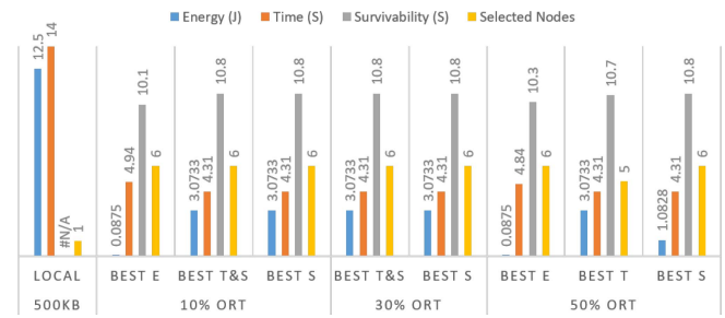
Fig. 9. Evaluation of our proposed solution in an ad hoc vehicular fog composed of four critical, three moderate, and four idle nodes while varying the nodes ORT using a 500-kB file.
